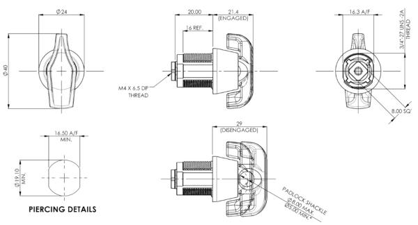
\*MINIMUM PADLOCK SHACKLE DIAMETER BASED ON 20mm INTERNAL SHACKLE RADIUS
