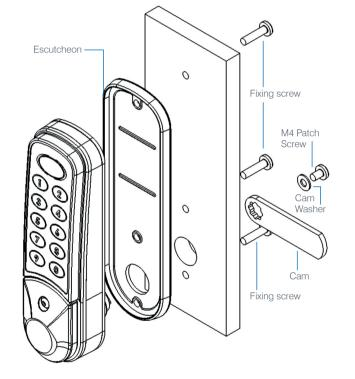
Holes **A**, **B** & **C** diameter 4.5 / 5.0mm Hole **D** diameter 16.0 / 16.5mm Always use fixing hole **A** and either fixing hole **B** or **C** (or both) Recommended screw fixing torque 0.8NM
