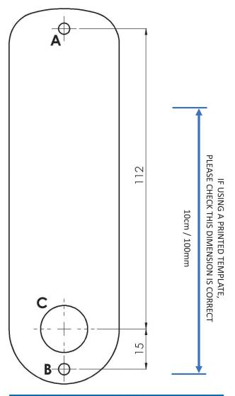
Holes **A** & **B** diameter 4.5 / 5.0mm Hole **C** diameter 17.0 / 17.5mm Recommended screw fixing torque 0.5Nm min.
