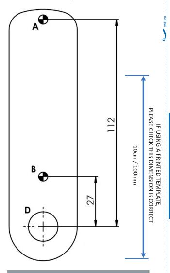
HOLES A, B & C DIAMETER 4.5 / 5.0mm HOLE D DIAMETER 16.5 / 17mm ALWAYS USE FIXING HOLE A and B
